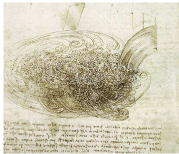
FIGURE 37.2. Mixing and emergence of organized structures in turbulent flow according to Leonardo da Vinci.
