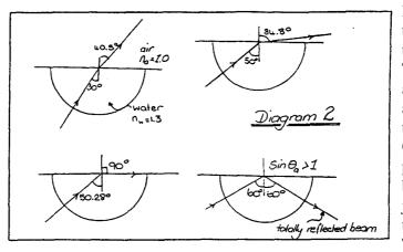
notice that they can see a reflection of the bottom of the pool on the top of the water, if they look at the surface at an angle of greater than about 50 degrees. Also they can see out of the pool, by looking up at an angle of less than that.
